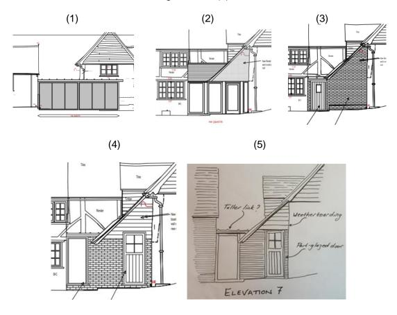
2.2 Whilst there would be a modest amount of harm occasioned to the farmhouse and to the East Stables by forming this link, this element is crucial to the accessibility of this courtyard group. The latest version follows the format offered in a sketch I prepared previously (see 5 above) and I am prepared to support this alteration.
