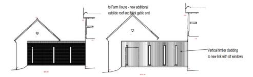
4.3 In light of comments previous made, the fenestration to both gable ends has been adjusted and is considered acceptable.
